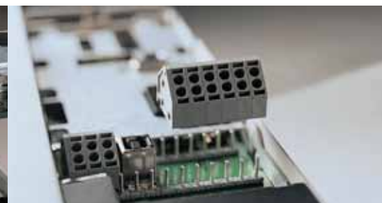
The fieldbus option ready to plug in beneath the front panel. It can be turned upside down if you'd rather have the cable on top.
