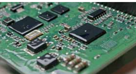
Coated control boards are available for harsh environments.
